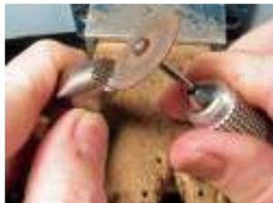
The tool I like to use to grind the pattern is a thin separating disc in a Foredom or Dremel. Be sure to hold the hammer and separating disc steady as you carve, and wear those safety glasses to protect your eyes.
